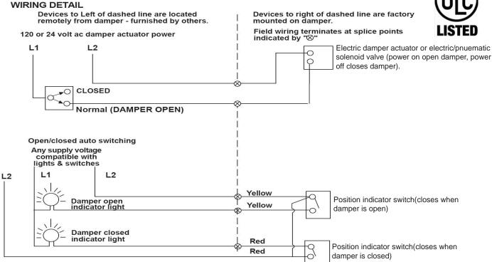
Detailed wiring diagrams including terminal designation and/or wire color coding furnished with each shipment.
