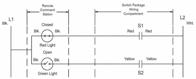
L1, L2 is a Supply Voltage Compatible with Lights and Switches. Standard Voltage is Same as Actuator Ordered.
